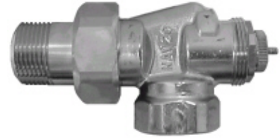
Horizontal angle valve with straight nipple. NPT - female inlet, male union outlet. 1/2" - N10837 3/4" - N10857 1" - N10877 1-1/4" - N10897
